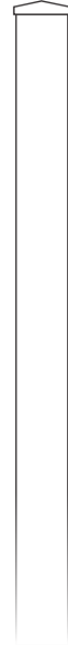
3" x 3" x 7' Aluminum post Qty: 6 Painted with peak cap Mount 2' below grade
