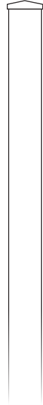
3" x 3" x 6' Aluminum post Qty: 8 Painted with peak cap Mount 2' below grade
