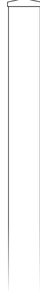
4" x 4" x 10' Aluminum post Qty: 12 Painted with peak cap Mount 2' below grade
