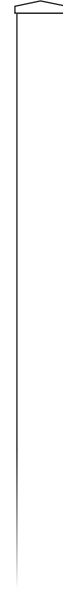
3" x 3" x 8' Aluminum post Qty: 10 Painted with peak cap Mount 2' below grade
