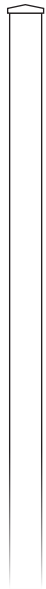
2" x 2" x 5' Aluminum post Qty: TBD Painted with peak cap Mount 2' below grade
